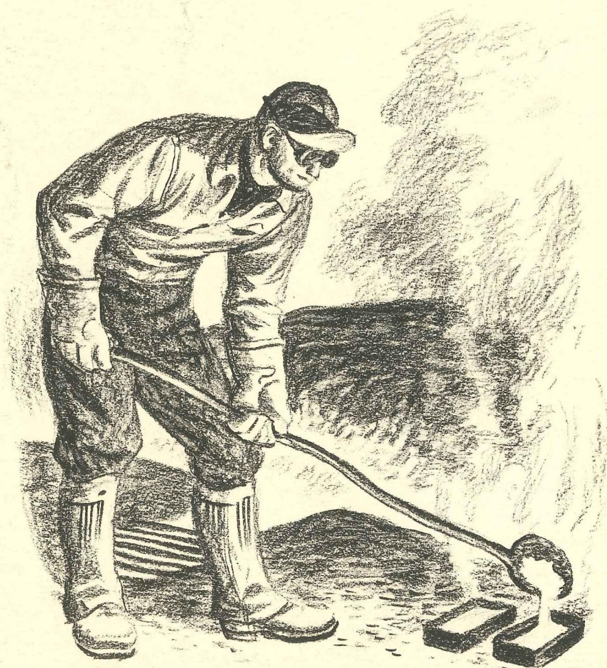
Workman hand-casts an iron sample for use by the laboratory
