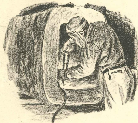
Cleaning an ingot mold on the chipping rack
