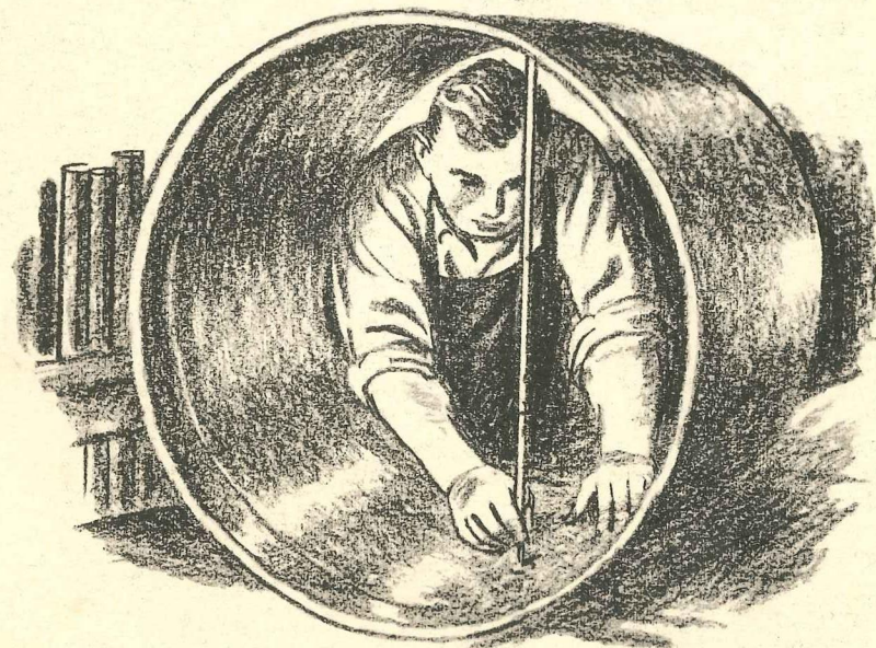
Final test measuring of a large centrifugal casting
